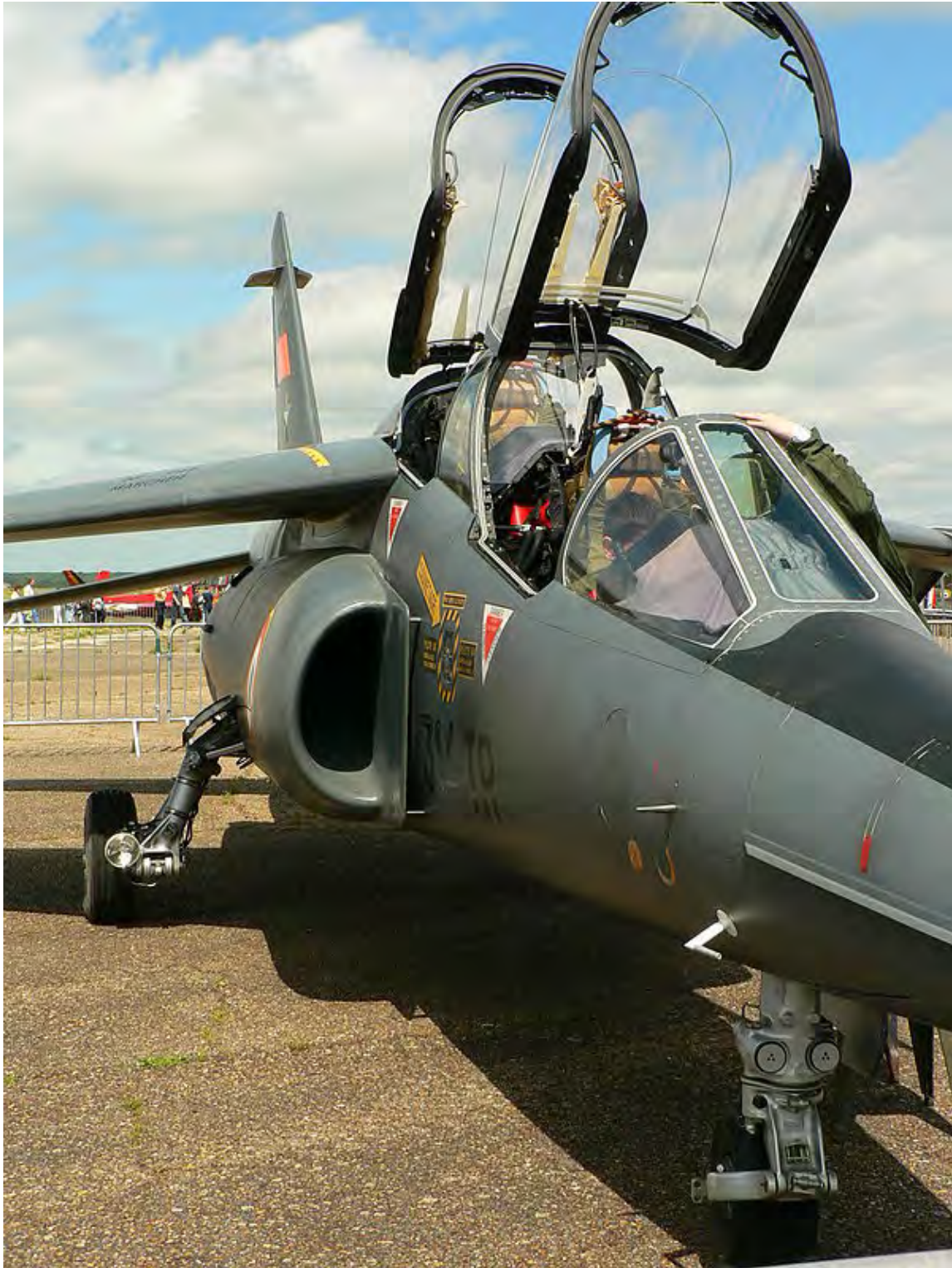
Duct work on an Dassault/Dornier Alpha Jet — At subsonic speeds, the increasing diameter of the inlet duct slows incoming air, causing its static pressure to increase.
