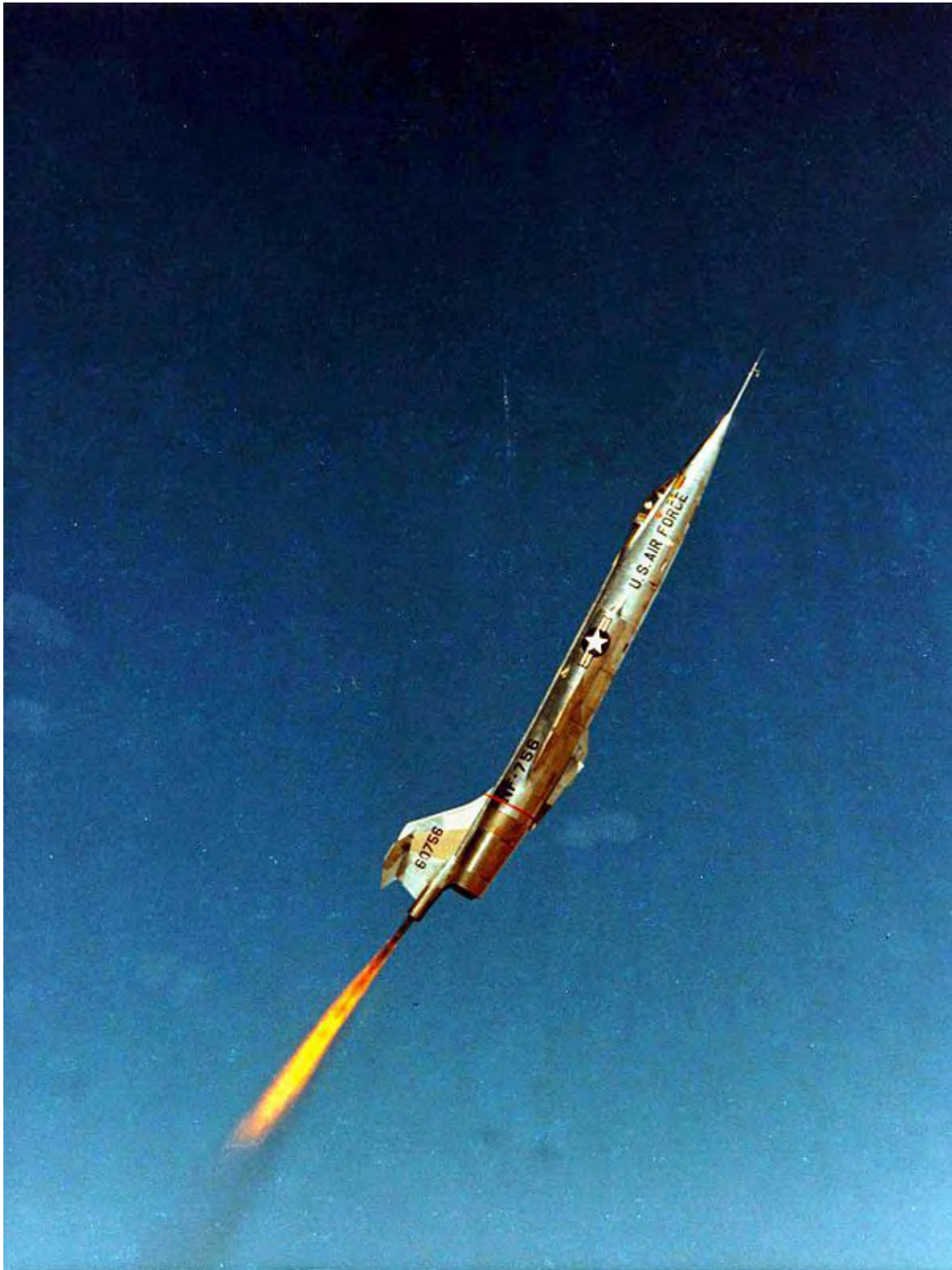
The Lockheed NF-104A had rocket and air-breathing turbojet engines, shown here climbing with rocket power. The rocket used hydrogen peroxide and JP-4 jet fuel.
