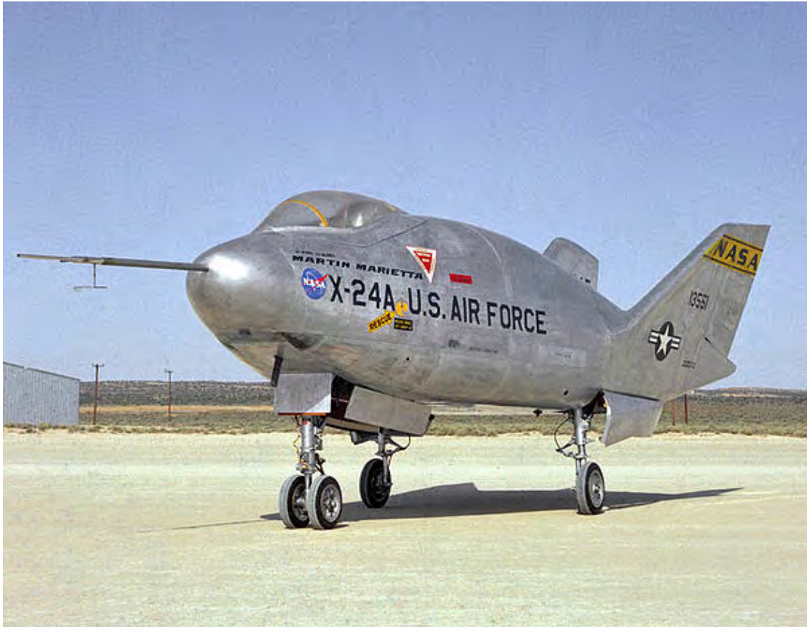
The Martin Aircraft Company X-24 lifting body built as part of a 1963 to 1975 experimental US military program
