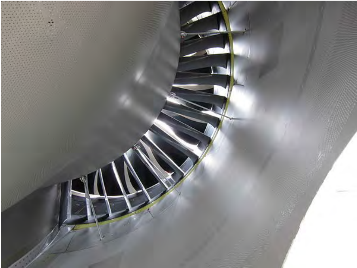
View into the outer (propelling or "cold") nozzle of a GEnx-2B turbofan engine
