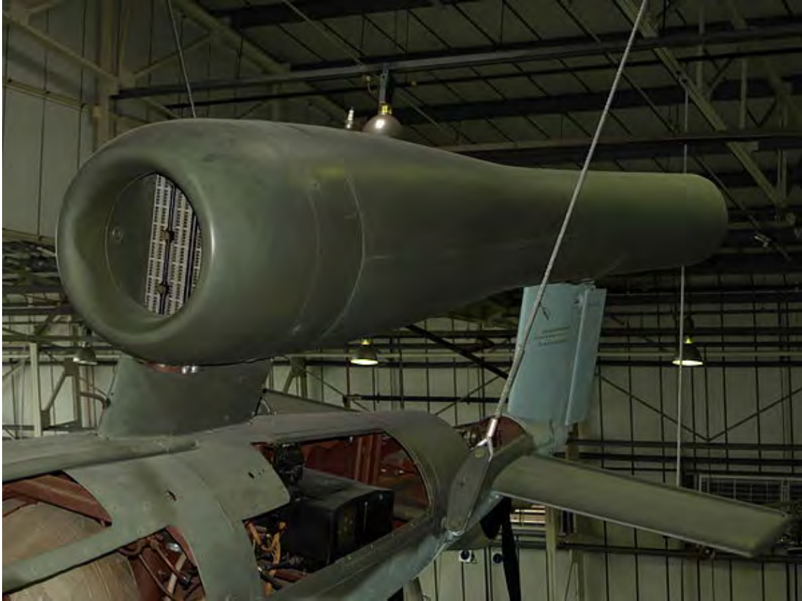
Argus As 014 pulse jet engine of a V-1 flying bomb at the Royal Air Force Museum London
