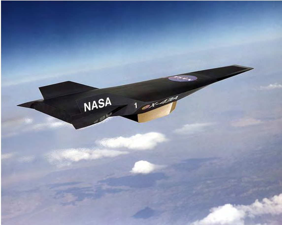
Artist's conception of the NASA X-43 with scramjet attached to the underside
