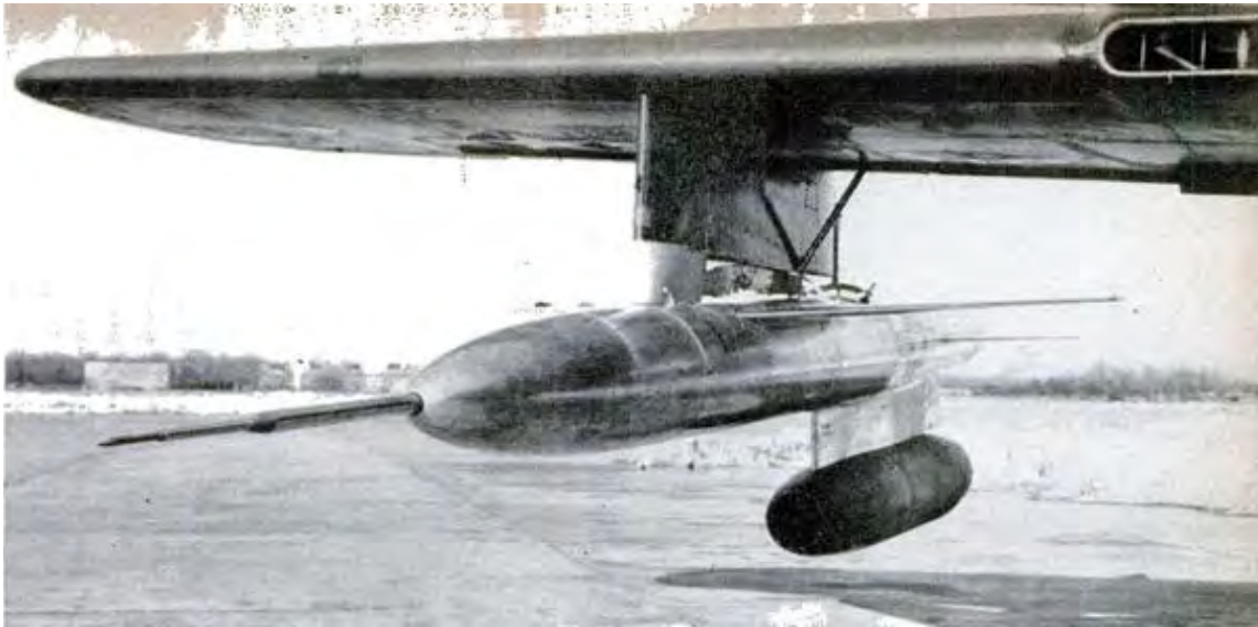
The Gorgon IV mounted on the wing of a P-61 Black Widow in preparation for flight testing
