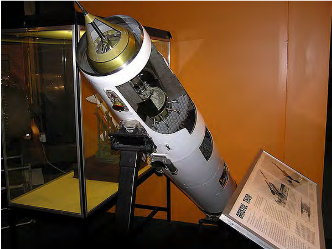
One of the two Bristol Thor ramjet engines on a Bristol Bloodhound missile
