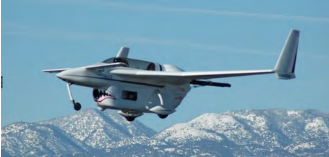
In-flight picture of the pulsed detonation powered, and heavily modified, Rutan Long-EZ on January 31, 2008.
