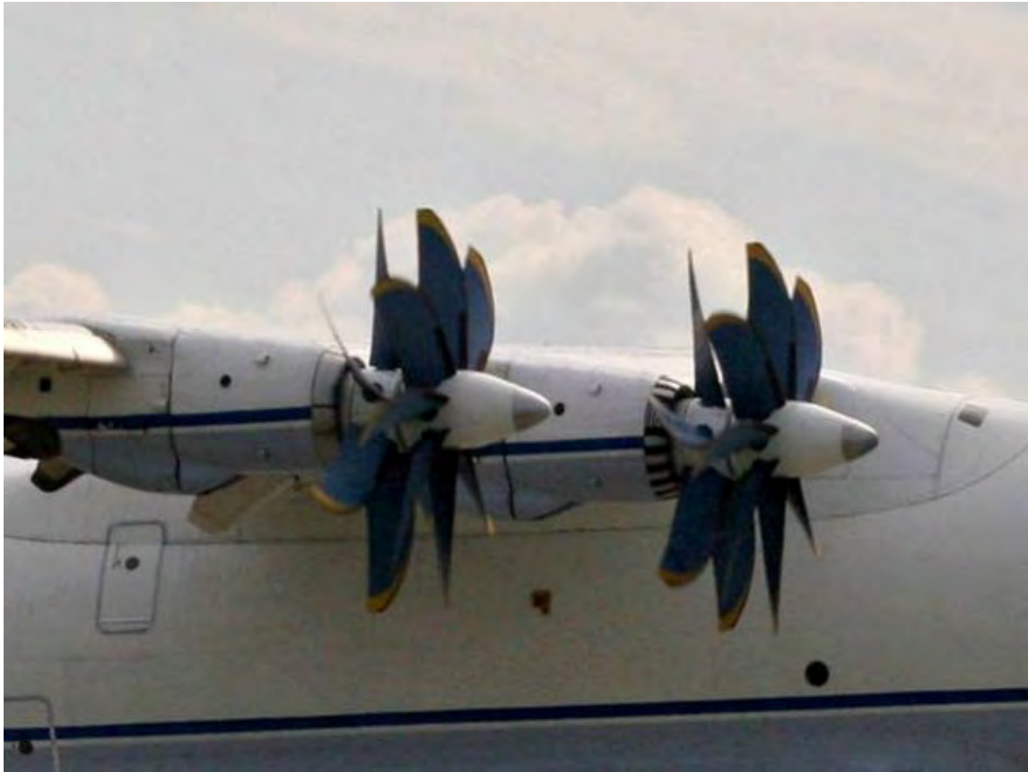
Progress D27 Propfans fitted to an Antonov An-70
