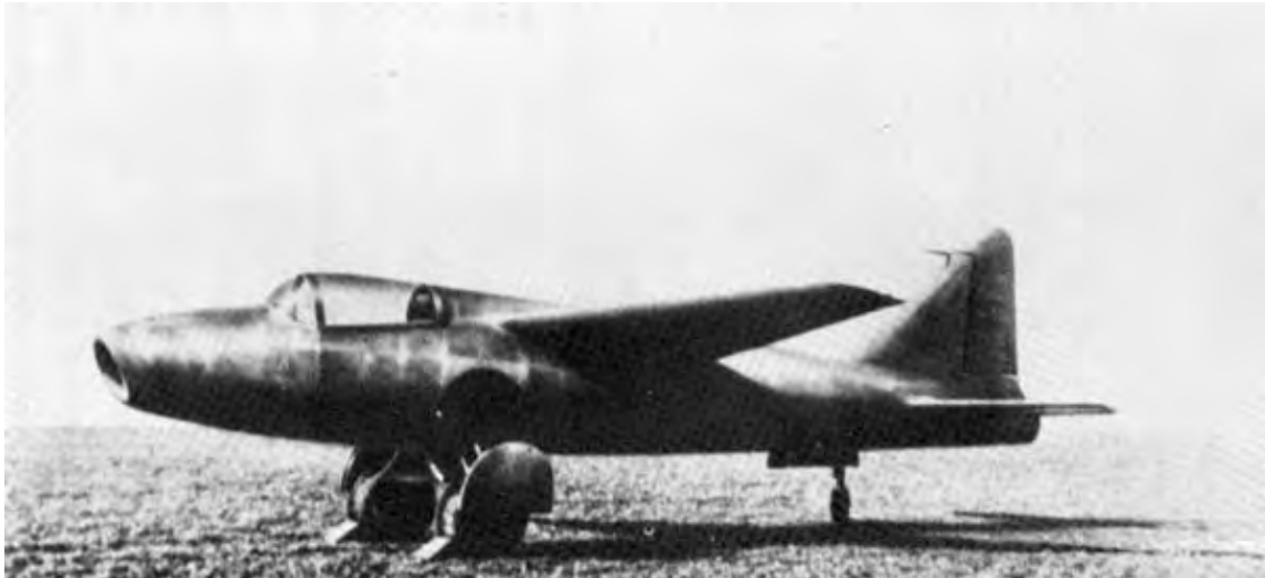
Heinkel He 178, the world's first aircraft to fly purely on turbojet power, using an HeS 3 engine
