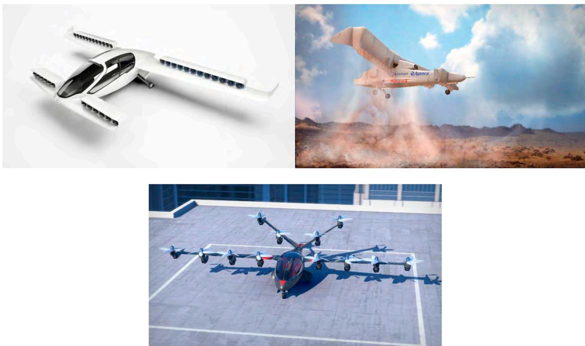
**Figure 1.** Vectored thrust electric vertical take-off and landing aircrafts (eVTOLs): Lilium Jet [13], Aurora Lightning Strike [23], Joby S2 [24].
