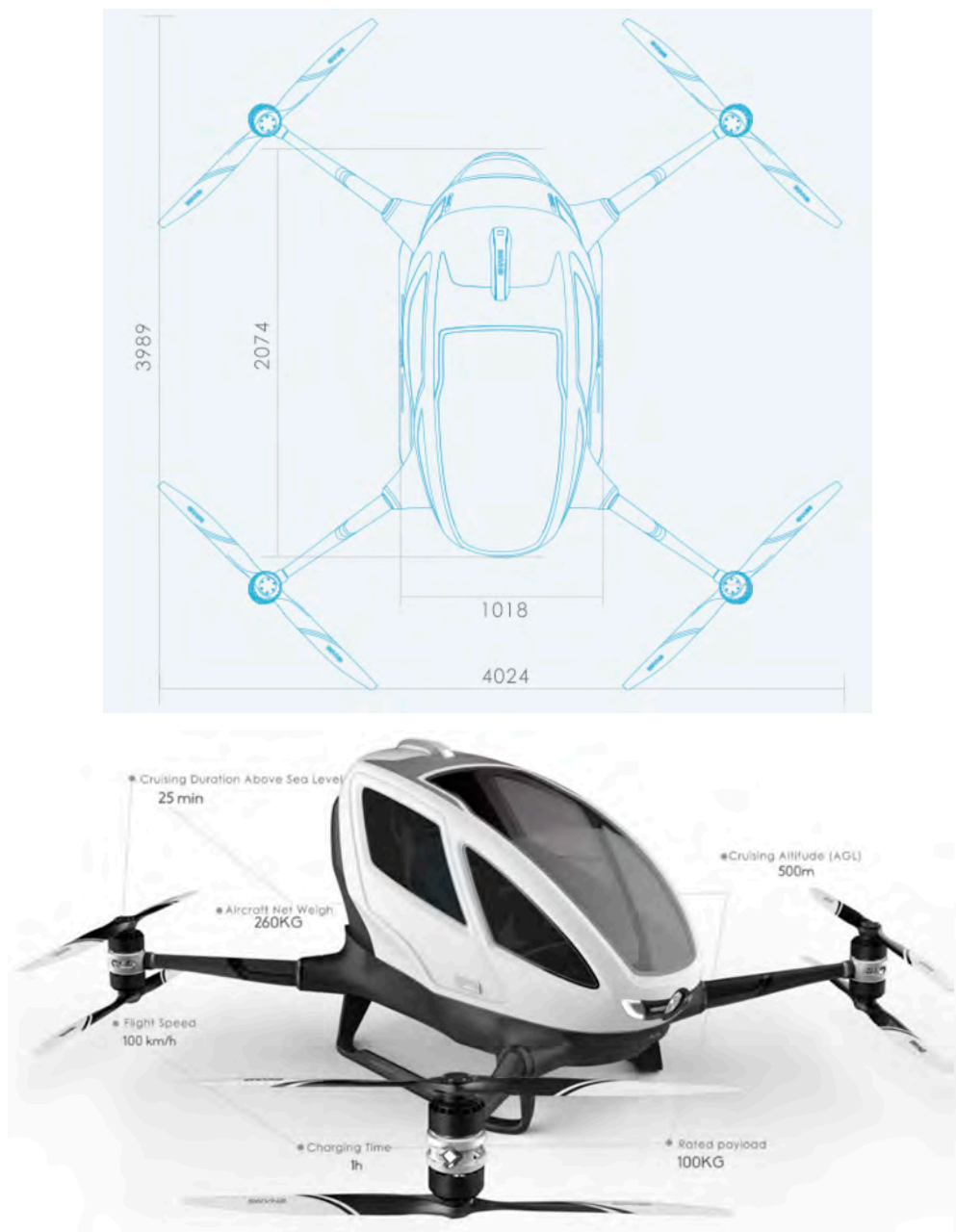
Figure 6. E-Hang 184 specs and dimensions, from E-Hang website [15]. Dimensions in the top view are in millimeters.
