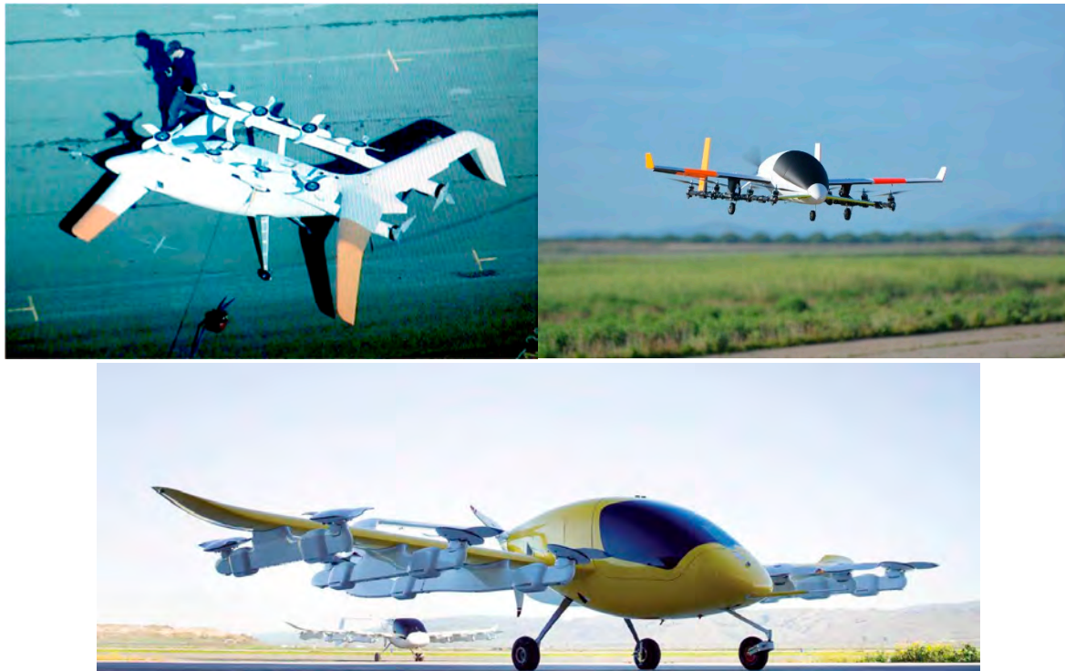
Figure 2. Lift + cruise eVTOLs: ZeeAero Z-P2 [25], Aurora Flight Sciences eVTOL [26], Kitty Hawk Cora [27]:
