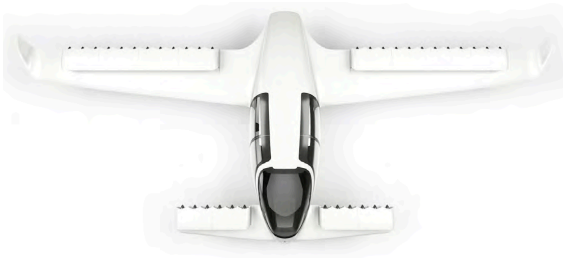
Figure 9. Lilium jet five-seater geometry.
